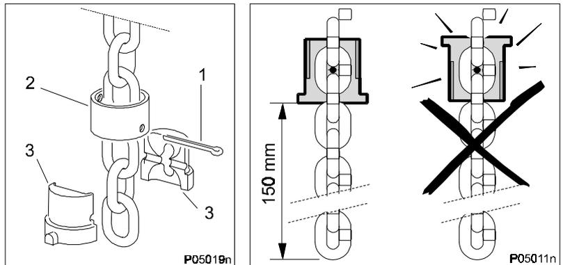
**Note:** Make sure that the stop is correctly fitted. The locking tube should be turned towards the hoist.
