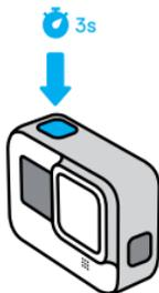
2. Press the Shutter button
