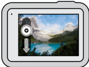
*Heads Up:* Some digital lenses only work with select frame rates. If needed, HERO8 Black will automatically adjust the frame rate when you switch lenses.
