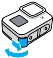
2. With your camera off, insert the SD card into the card slot with the label facing the battery compartment.
