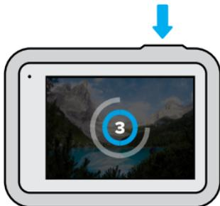
*Heads Up:* To help prevent blurry low-light shots, the timer is automatically set to 3 seconds when you switch to Night photo mode.
