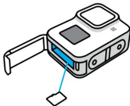
You can eject the card by pressing it into the slot with your fingernail.
