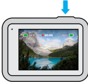
2. Press the Shutter button
